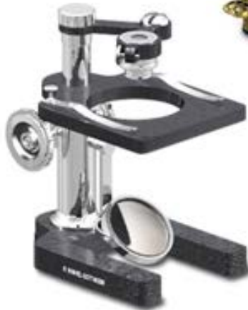
Winkel-ZEISS Dissecting Microscope (circa 1927)
